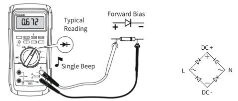
Remove all the terminals of the inverter PCBA before check.
