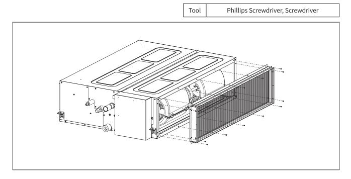
(4) Remove M4 screw (Quantity: B) that is fixing the lower back cover to the indoor motor side. Remove the lower back cover.
