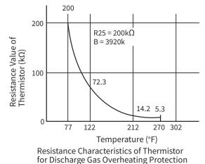
(d) If compressor upper part temperature increases excessively, the protection control is activated and the compressor forced frequency reduction according to the following method.
