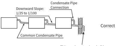
This condensate pipe shall be separating from other pipes.
