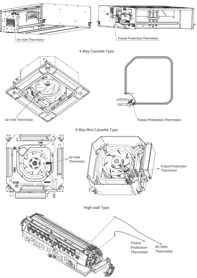
(2) Thermistor for Indoor Suction Air Temperature (For Room Temperature Control)
