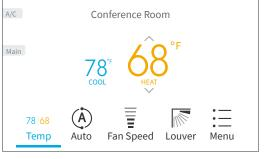
If the condition of "cooling setpoint ≥ heating setpoint +3°F" is not satisfied, setup is unavailable.
