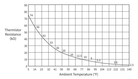
Ambient and Evaporating Temp. Thermistor Characteristics for Outdoor Unit
