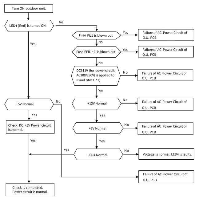
\*1) The following table shows the check points and the normal range of voltage in the case that the voltage on O.U. PCBA is measured by a digital multimeter. The setting of digital multimeter shall be set within the DC voltage measurement range when the following voltages are measured.
