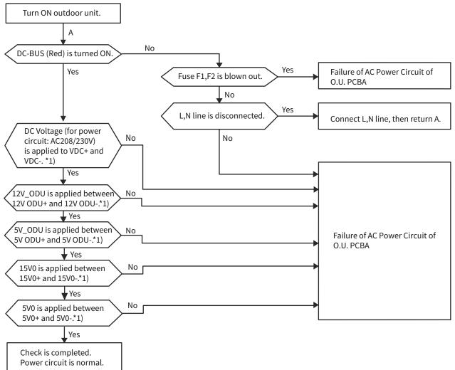
\*1) The following table shows the check points and the normal range of voltage in the case that the voltage on O.U. PCBA is measured by a digital multimeter. The setting of digital multimeter shall be set within the DC voltage measurement range when the following voltages are measured.
