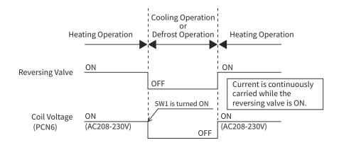
(4) Output Voltage of PCN6 on PCB1
