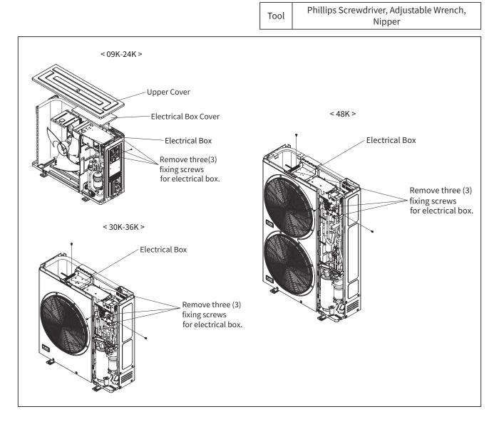
Remove the electrical box after disconnecting wires.
