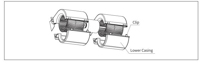
(9) Use hexagonal wrench to remove the M6 screw (1 pc per fan) that is fixing the fan. Remove the fan from the motor shaft in the direction shown by the arrow in the figure.
