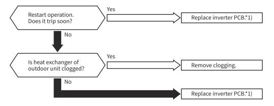
\*1) The maintenance and replacement for inverter PCB should be performed after performing surely the voltage discharge work according to the item 1.2.4 (2) "Checking Method for Rectifier Circuit".
