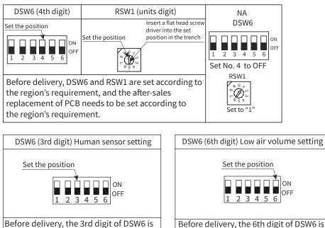
set to "0". Set the 3rd digit of DSW6 to "1" when installing human sensor.
