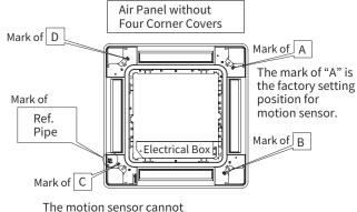
The motion sensor cannot install to the location of the mark of "C".
