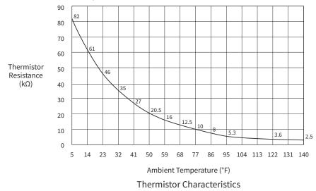
Economical Cooling Operation: 80°F to 84°F / Economical Heating Operation: 64°F to 68°F The resistance characteristics of thermistor is shown in the above figure.
